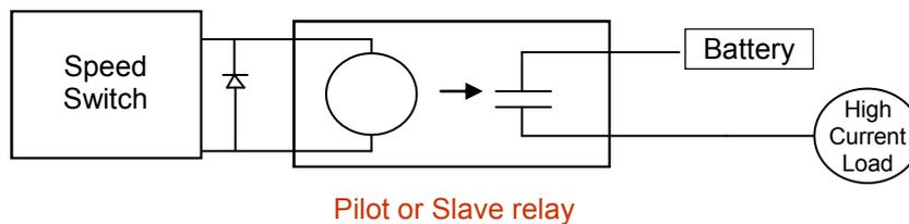
The Pilot or Slave relay simply “relays” the signal to the high current load. The input to the Slave relay can be small but it can control currents up to 100’s of amps. A diode is shown in the above illustration. This is a low cost preventative that adds years of useful life. The diode channels the surges of the slave relay into a harmless dissipation as opposed to causing arcing in the control contacts of the engine control.
