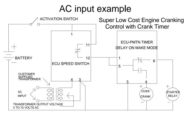
SS21 Speed switch AC transformer operation
